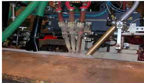
Fig 1. SAW or submerged arc welding equipment completing a weld. The weld starts on the right and moves left. The gray colored powder is flux.
