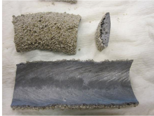
Fig 2. Pieces of slag from Submerged arc welding
